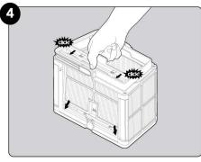
Assemble the filter panels.
